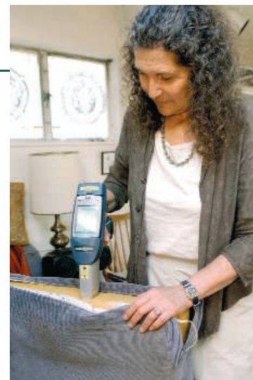
Detection. Biophysical chemist Arlene Blum, using an x-ray fluorescence analyzer, measures 5% bromine from the fire retardant in her couch foam.
