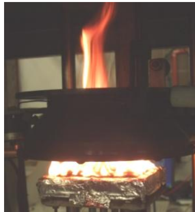
Combustion Cone Calorimeter+ FTIR analysis
